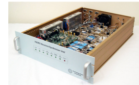
Receiver/Synthesizer Unit – NOAA Severe Storm Airborne Radar
